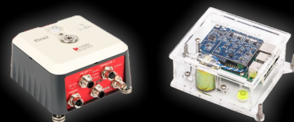
Examples of accelerometers deployed by INFP for structural monitoring: Etna2 (Kinematics) or 4D (RaspberryShake).
